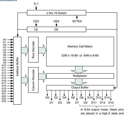
are placed in a high-Z state and pin D15 functions as the A-1 address pin.
